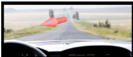
Fig. 2. In-car Augmented Reality: Guiding driver's attention to dangerous situation. The arrow indicates the position of imminent danger (from [6]).
